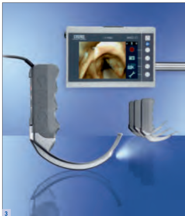
The new videolaryngoscope C-MAC® (KARL STORZ Tuttlingen, Germany) provides a clear image of the glottic inlet, with vocal cords, arytenoids and surrounding area. User-friendly pushbuttons on the monitor allow users to control a multitude of functions, such as video recording, still image capture, automatic white balancing and image focusing, brightness and contrast adjustment.
